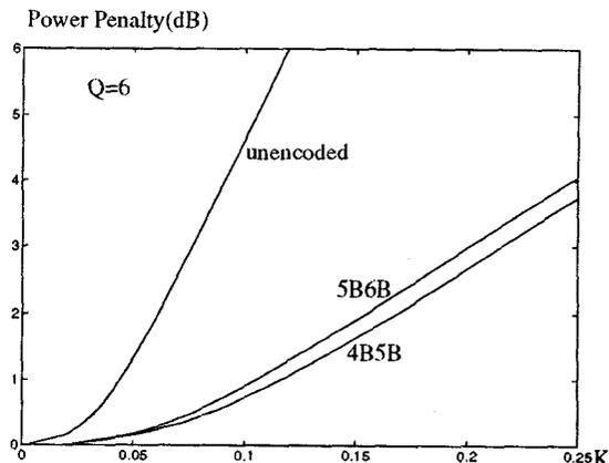
Fig. 3 Power penalty versus decay parameter  $K$  for input data.
