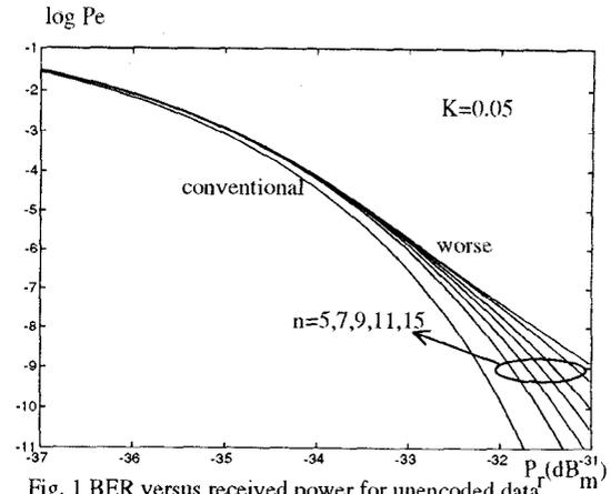
Fig. 1 BER versus received power for uncoded data.
