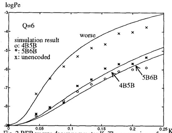
Fig. 2 BER versus decay parameter  $K$ . The comparison of simulation results and theoretical results (solid line)
